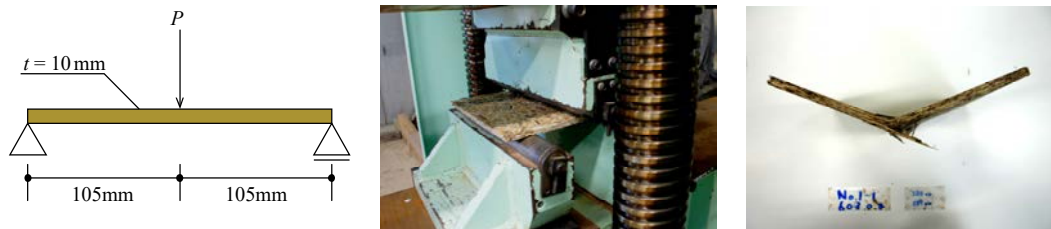
Figure 6: Bending test condition (left and middle) and failure situation after test of S1 (right)
